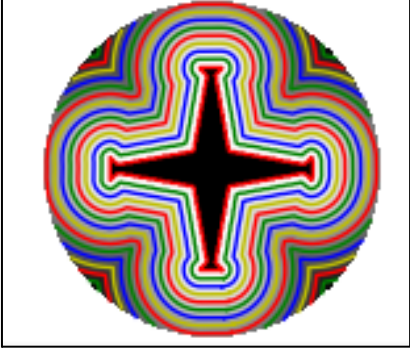
Figure 46: Fuel grain burn contours, simulated in Openmotor
