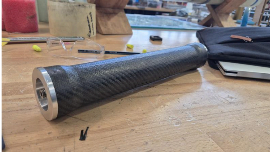
Figure 49: Final cured 60mm Test Article 1, showing surface conditions and overall geometry
