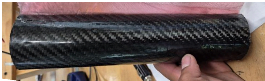
Figure 50: damaged composite structure from test article 2
