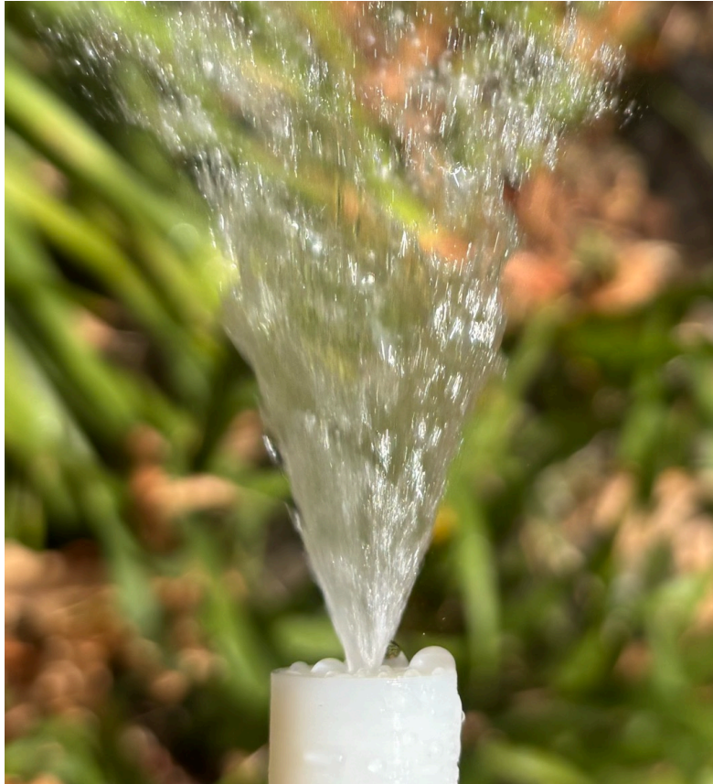
Figure 8: One test of a 3D printed swirl injector.
