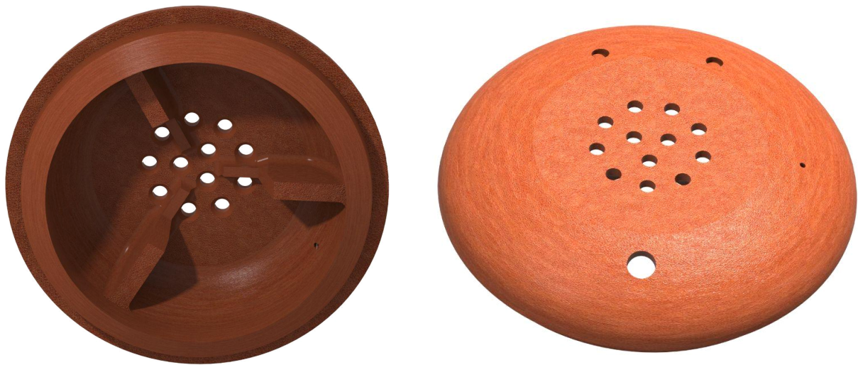
Figure 29: Render of swirl injector pre-combustion chamber
